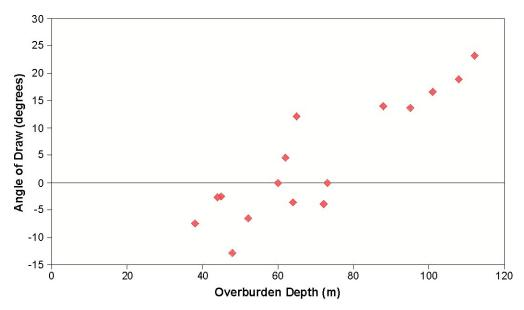
Figure 10 Relationship between angle of draw measured at Ashton and overburden depth.
