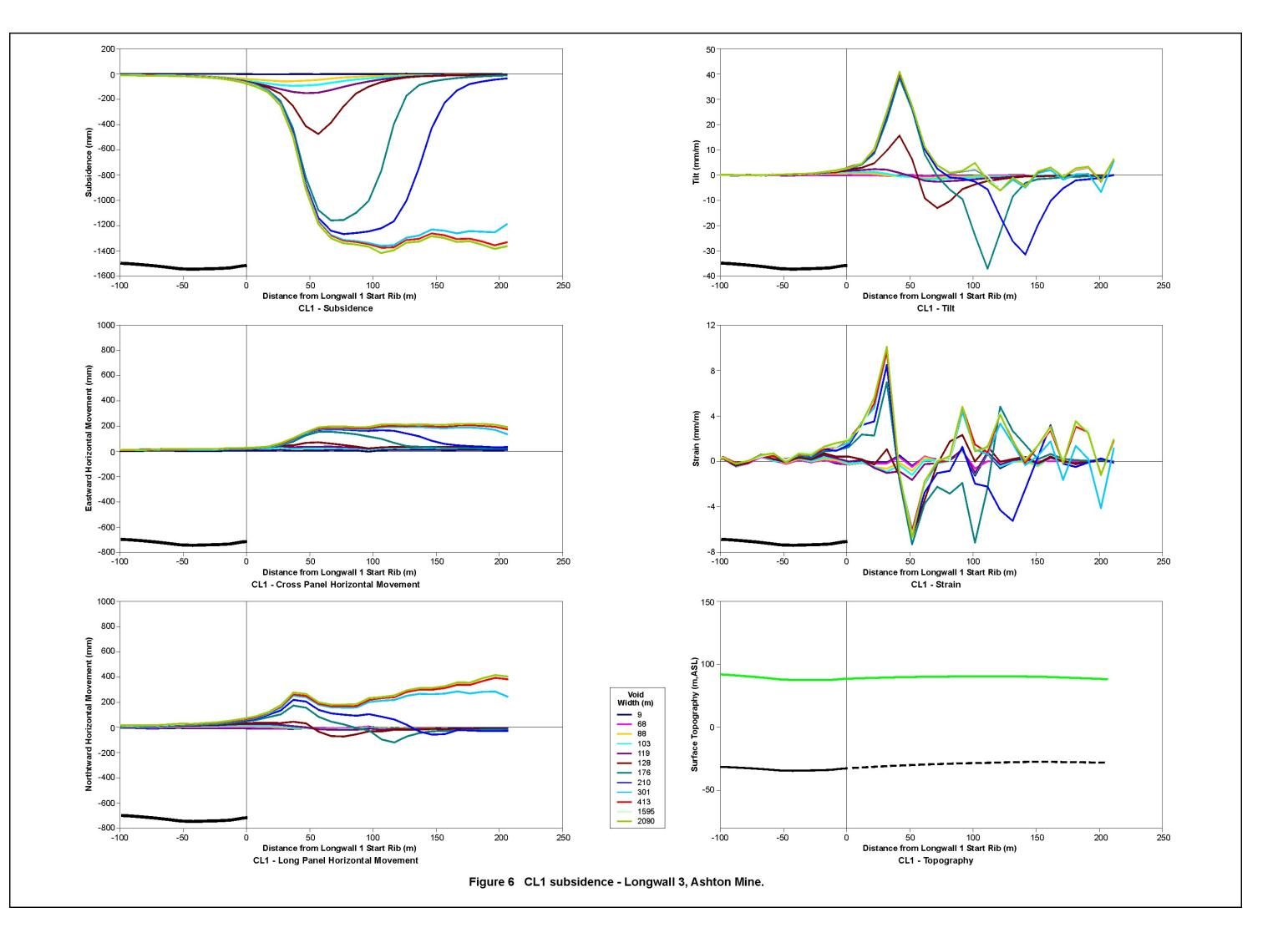
movement was toward the void and then a reversal occurred leaving a final offset in the direction of mining of up to 276mm near the start of the panel and a peak horizontal movement in the direction of mining of approximately 415mm. The horizontal movements extended back over the solid starting rib to the end of the line where they were still 15mm at 113m from the goaf edge.
