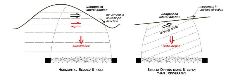
Figure 8 Sketch illustrating the mechanics of horizontal movement.
