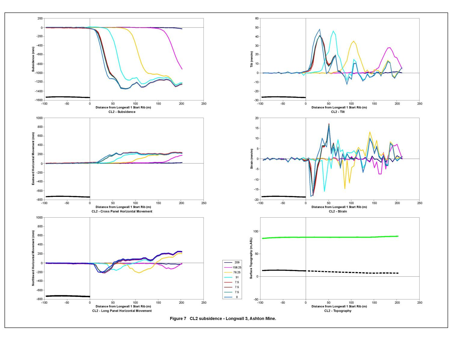
In general the subsidence movements measured are less than predicted, except for the tensile strains at the start of Longwall 1 measured on CL1, which were 49mm/m compared to the 42mm/m maximum predicted and the maximum tilt on XL5 above Longwall 3, which was 97mm/m compared to the predicted maximum 78mm/m.
