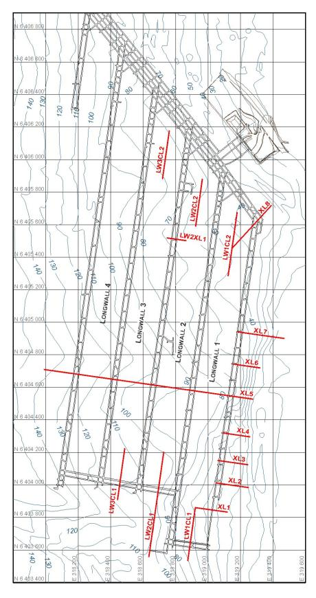
Figure 2 Overburden depth to the Pikes Gully Seam.
