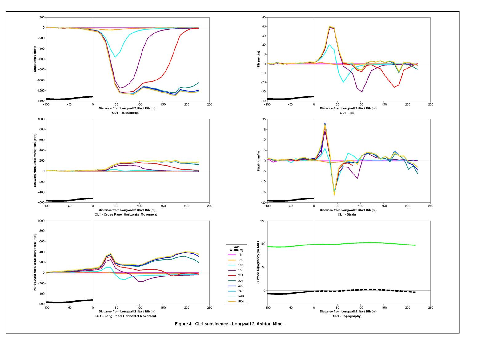
450mm. The horizontal movements extend back over the solid starting rib approximately 100m, or a distance equal to the overburden depth.
