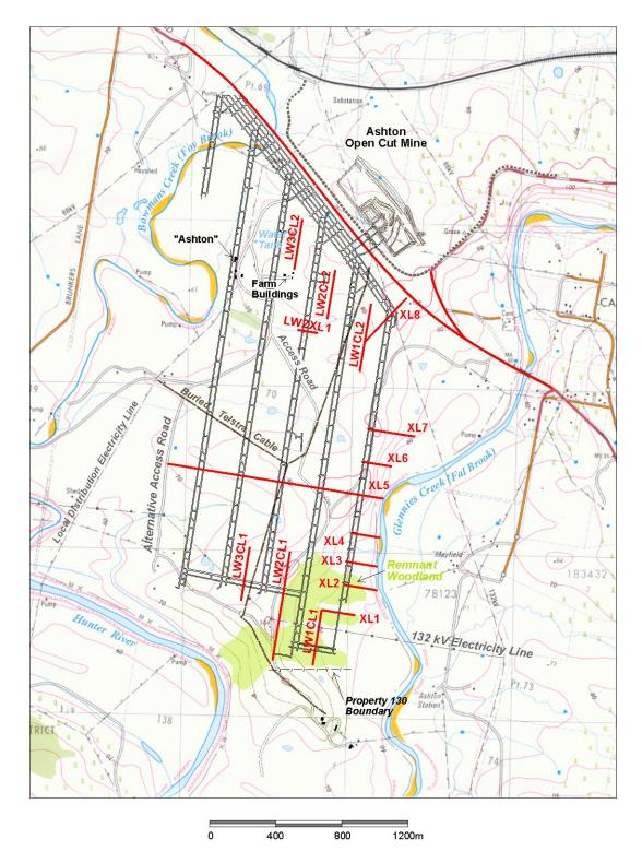
Figure 1 Site plan showing mine plan and location of the subsidence lines superimposed onto 1:25,000 topographic series map updated to reflect current infrastructure.
