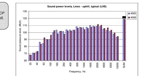
FIGURE 3 Sound power levels of ACP haul trucks travelling uphill, loaded.
