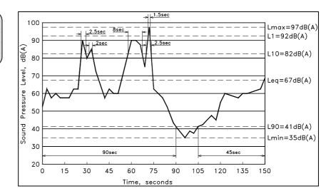
The signal in Figure 2 has a duration of 2.5 minutes (ie 150 seconds) with noises occurring as follows:
