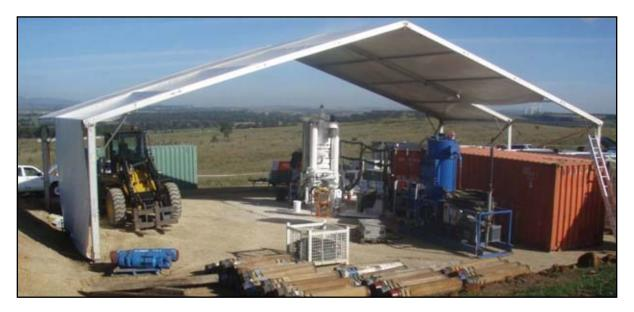
Photograph 2: Typical raise bore drilling rig and temporary marquee (source: ACOL)
