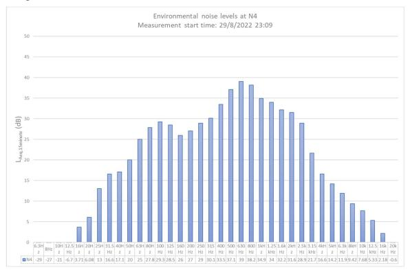
Figure 5.3 N4 total measured one-third octave band frequencies
