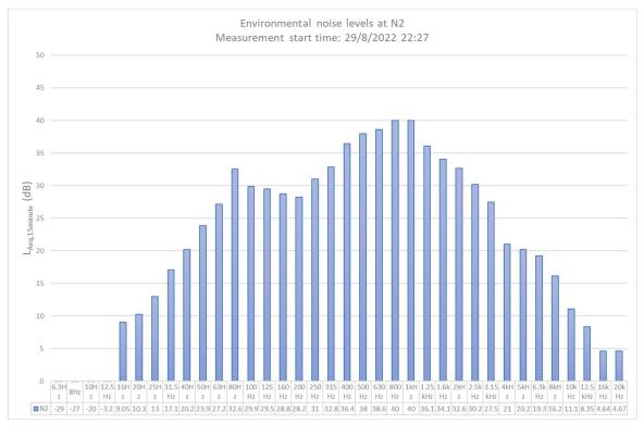
Figure 5.1 N2 total measured one-third octave band frequencies
