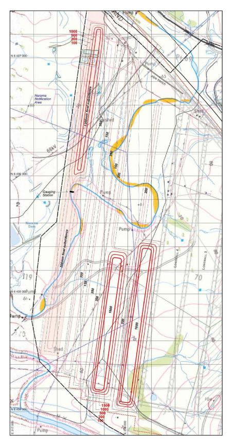
Figure 6: Final predicted subsidence contours
