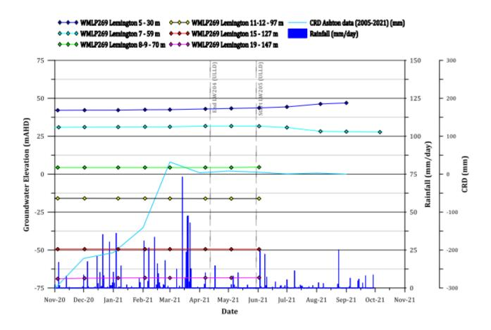
\* WMLP 269 – Vibrating Wire sensors from 70m to 147m returned erroneous results.
